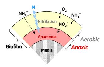
This can be achieved within a single MBBR reactor. Specific conditions (pH, temperature, oxygen level) are maintained within the reactor to allow the process specific bacteria to grow as a biofilm on AnoxKaldnes carrier media. All the benefits of proven MBBR technology are applicable to ANITA<sup>™</sup> Mox including retention of critical biomass, a stable and robust process and a small footprint.
